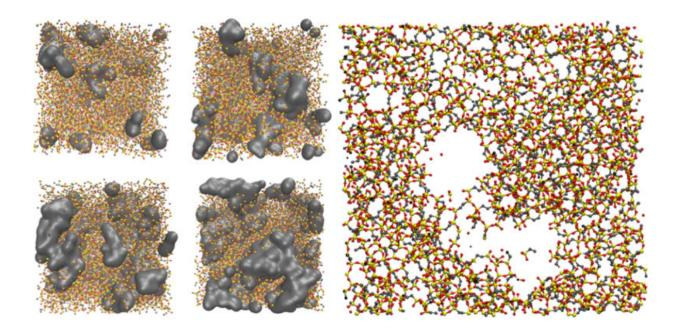
In modeling new protective materials, the researchers introduced sacrificial molecules (shown in grey) in the four-frame simulation on the left. These molecules can be removed after the material is made, leaving behind tiny pores (visible in the larger frame on the right) that make the material more durable to expansion and contraction. Credit: Dauskardt Group
