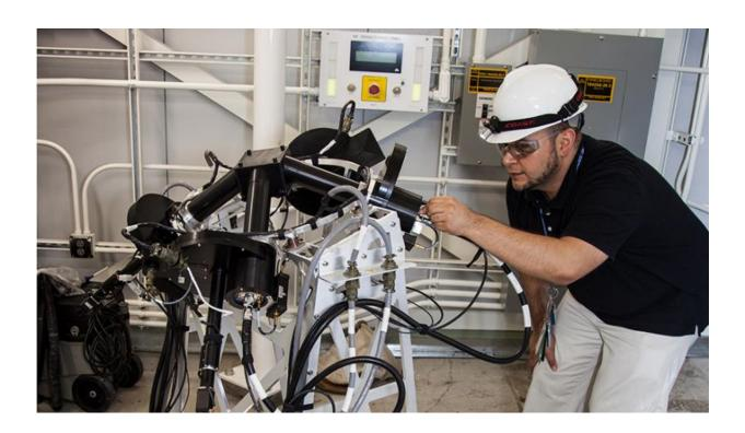
Target Diagnostics engineer Francisco Barbosa completes installation of the North Pole neutron Time of Flight (nTOF) diagnostic on the roof of the National Ignition Facility. Credit: Lawrence Livermore National Laboratory
