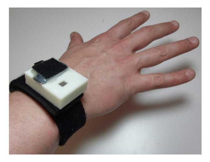
An early prototype of the wristband used in the Health and Environmental Tracker (HET), an integrated, wearable system that monitors a user's environment, heart rate and other physical attributes with the goal of predicting and preventing asthma attacks. Credit: James Dieffenderfer
