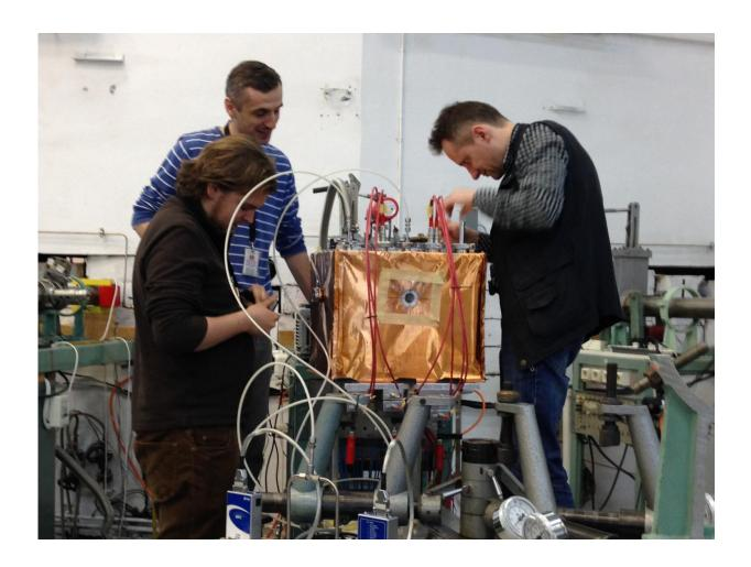
This image shows the installation of the mini-eTPC demonstrator detector during on-line test beams at the 9 MV Tandem accelerator facility at IFIN-HH, Magurele, Romania. From left: Jan Stefan Bihalowicz, Lukasz Janiak, Marcin Zaremba. Credit: Faculty of Physics, University of Warsaw
