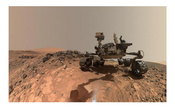
This low-angle self-portrait of NASA's Curiosity Mars rover shows the vehicle at the site from which it reached down to drill into a rock target called "Buckskin." Bright powder from that July 30, 2015, drilling is visible in the foreground. Credit: NASA/JPL-Caltech/MSSS
