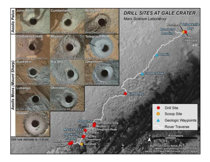
This graphic maps the first 14 sites where NASA's Curiosity Mars rover collected rock or soil samples for analysis using the rover's onboard laboratory. It also presents images of the drilled holes where 12 rock-powder samples were acquired. At the other two sites Curiosity scooped soil samples. Credit: NASA/JPL-Caltech/MSSS
