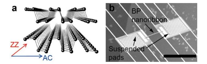
Thermal properties (as measured via the experimental set-up on the right) of a black phosphorus nanoribbon were a factor of two different along two directions in the crystal structure (image on the left). Specifically, the zig-zag (ZZ) direction was two times more conductive than the "arm chair" (AC) direction. Credit: Junqiao Wu, University of California-Berkeley/Nature Communications
