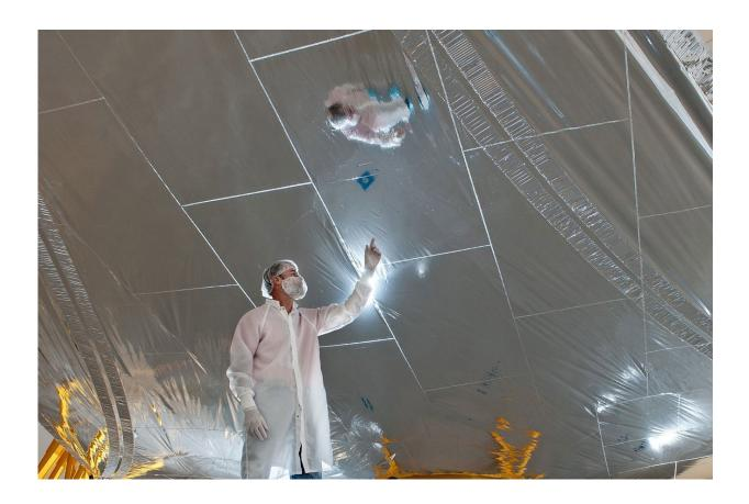
An engineer in a cleanroom looks at one of the sunshield layers that shows a grid pattern of "rip-stops." Credit: Nexvolve
