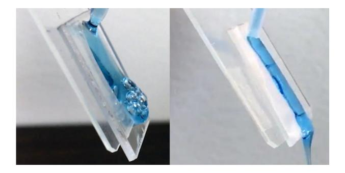
Laundry detergent spreads out on a piece of normal polycarbonate (left), but flows off a piece of treated polycarbonate in a steady stream (right). Engineers at The Ohio State University have invented a coating that lets soap flow out of plastic bottles more easily. Credit: Philip S. Brown, courtesy of The Ohio State University.
