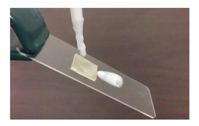
Engineers at The Ohio State University have invented a coating to help soap pour out of plastic bottles more easily. Here, a drop of shampoo slides off a piece of polypropylene. Credit: Philip S. Brown, courtesy of The Ohio State University.
