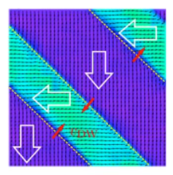
Once domain walls are established, they move across the material as domains aligned with the external electric fields grow. Credit: University of Pennsylvania
