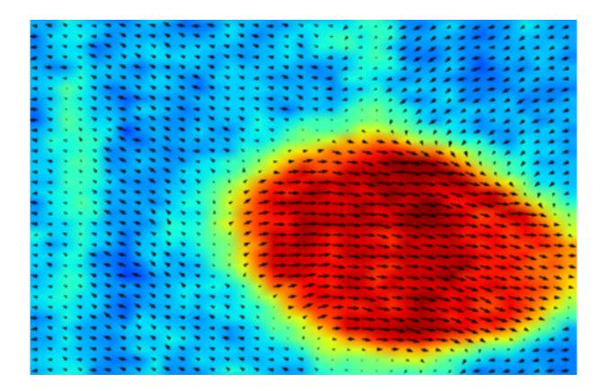
The simulations show that thermal fluctuations are responsible for the first nuclei from which changes in polarization spread. Credit: University of Pennsylvania
