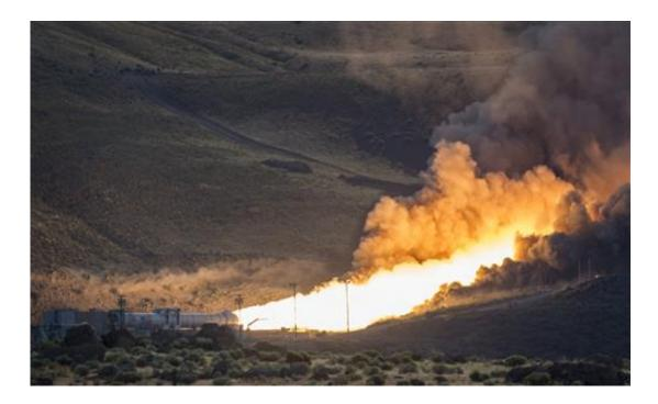
The second and final qualification motor (QM-2) test for the Space Launch System's booster is seen, Tuesday, June 28, 2016, at Orbital ATK Propulsion Systems test facilities in Promontory, Utah. During the Space Launch System flight the boosters will provide more than 75 percent of the thrust needed to escape the gravitational pull of the Earth, the first step on NASA's Journey to Mars. (Bill Ingalls/NASA via AP)
