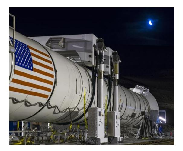
The moon rises ahead of the second and final qualification motor (QM-2) test for the Space Launch System's booster, Tuesday, June 28, 2016, at Orbital ATK Propulsion Systems test facilities in Promontory, Utah. During the Space Launch System flight the boosters will provide more than 75 percent of the thrust needed to escape the gravitational pull of the Earth, the first step on NASA's Journey to Mars. (Bill Ingalls/NASA via AP)
