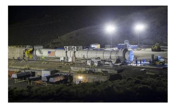
The Space Launch System's booster is seen a few hours ahead of the second and final qualification motor (QM-2) test, Tuesday, June 28, 2016, at Orbital ATK Propulsion Systems test facilities in Promontory, Utah. During the Space Launch System flight the boosters will provide more than 75 percent of the thrust needed to escape the gravitational pull of the Earth, the first step on NASA's Journey to Mars. (Bill Ingalls/NASA via AP)
