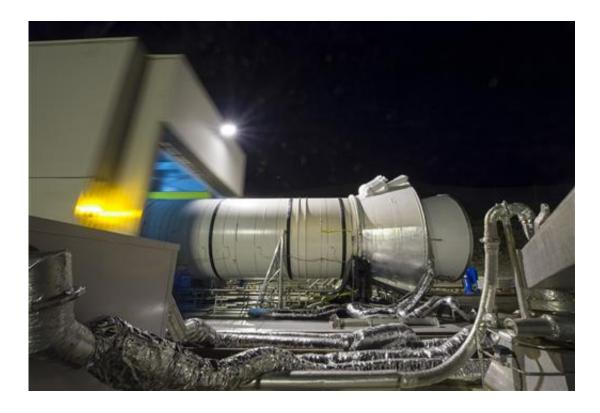
The booster house is rolled back ahead of the second and final qualification motor (QM-2) test for the Space Launch System's booster, Tuesday, June 28, 2016, at Orbital ATK Propulsion Systems test facilities in Promontory, Utah. During the Space Launch System flight the boosters will provide more than 75 percent of the thrust needed to escape the gravitational pull of the Earth, the first step on NASA's Journey to Mars. (Bill Ingalls/NASA via AP)
