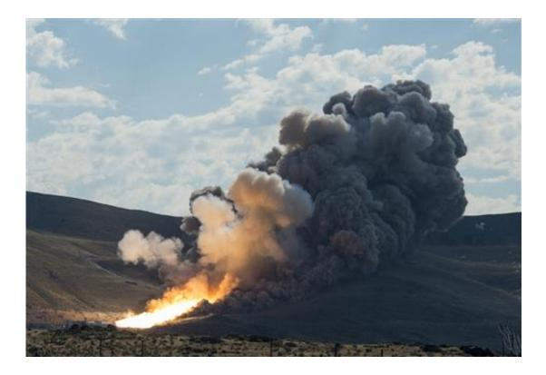
The second and final qualification motor (QM-2) test for the Space Launch System's booster is seen, Tuesday, June 28, 2016, at Orbital ATK Propulsion Systems test facilities in Promontory, Utah. During the Space Launch System flight the boosters will provide more than 75 percent of the thrust needed to escape the gravitational pull of the Earth, the first step on NASA's Journey to Mars. (Bill Ingalls/NASA via AP)
