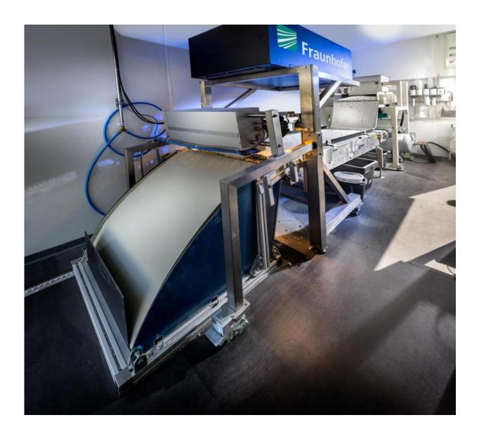
Sorting machine with conveyor belt, which transports the shredded plastic waste. Credit: Fraunhofer IOSB
