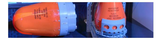
Professor David Stupples, City's Professor of Electronic and Radio Systems, says the time has come for the flight data recorder (FDR) and the cockpit data recorder (CDR) - the black box found on aircraft - to be stored in the cloud. The usually orange-coloured flight recorder is an electronic recording device used in the event of an aviation accident (or incident) investigation.
