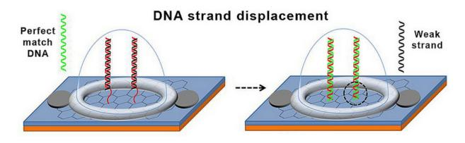
Schematic of DNA strand displacement on the biosensor chip. A perfect match DNA strand (green) binds to the normal strand (red) of the DNA probe and displaces the weak strand (black). Credit: Lal Research Group at UC San Diego
