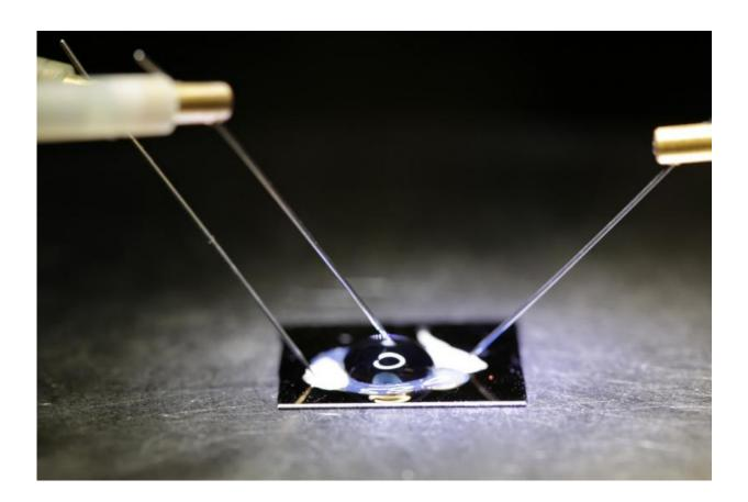
The biosensor chip—consisting of a double stranded DNA probe embedded onto a graphene transistor—electronically detects DNA SNPs. Credit: University of California - San Diego
