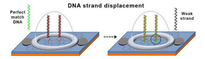
Schematic of DNA strand displacement on the biosensor chip. A perfect match DNA strand (green) binds to the normal strand (red) of the DNA probe and displaces the weak strand (black). Credit: Lal Research Group at UC San Diego
