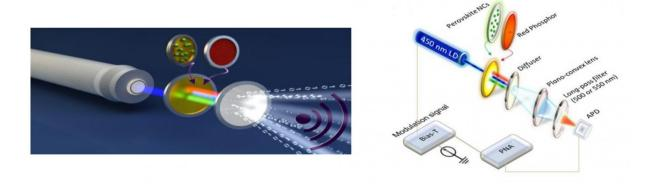
Illustration and schematic drawing of the visible light communication (VLC) device that uses a new color converter made of perovskite nanocrystals combined with red-light-emitting phosphor. Credit: Dursun et al. ©2016 American Chemical Society
