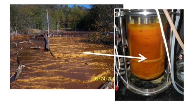
This research aims to translocate the natural process of biological low-pH iron oxidation into engineered bioreactors for more effective treatment of acid mine drainage. Penn State
