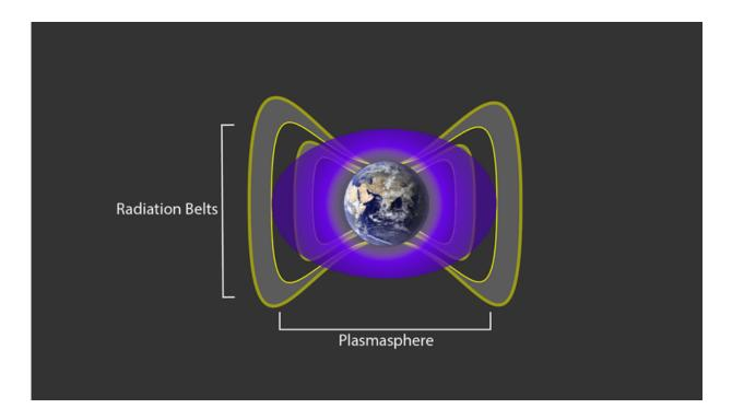
A cloud of cold charged gas around Earth, called the plasmasphere and seen here in purple, interacts with the particles in Earth's radiation belts — shown in grey — to create an impenetrable barrier that blocks the fastest electrons from moving in closer to our planet. Credit: NASA/Goddard
