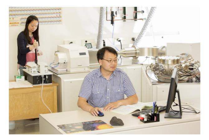
Co-authors Yan Hu (l) and Fang-Zhen Teng with the MC-ICP-MS machine (right) that turns basalt into a plasma, in which electrons are separated from each atom's nucleus, to discover tiny variations in the rock's chemical makeup. Credit: Dennis Wise/University of Washington
