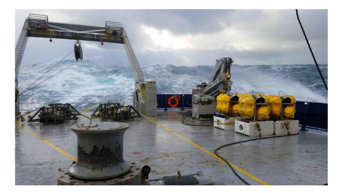
Seafloor absolute pressure gauges lashed to the deck of the R/V Roger Revelle. It's important to strap down the instruments, especially during high seas, such as those sometimes found offshore of Gisborne, New Zealand. Credit: Justin Ball, University of Colorado
