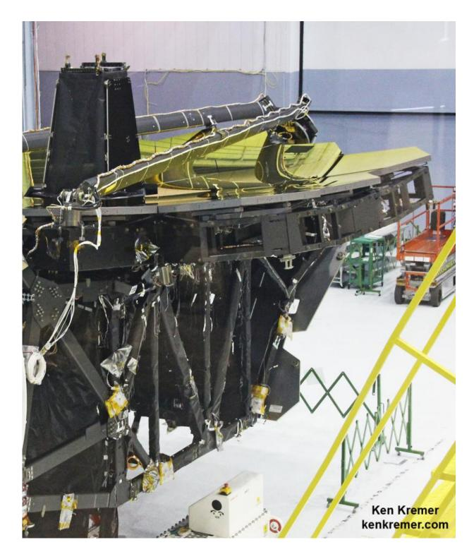
Up close view shows cone shaped Aft Optics Subsystem (AOS) standing at center of Webb telescopes 18 segment primary mirror at NASA's Goddard Space Flight Center in Greenbelt, Maryland on May 3, 2016. ISIM science instrument module will be installed inside truss structure below. Credit: Ken
