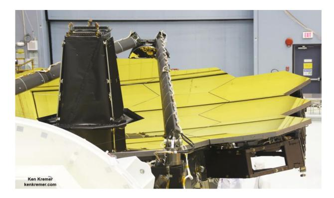
Up close side-view of newly exposed gold coated primary mirrors installed onto mirror backplane holding structure of NASA's James Webb Space Telescope inside the massive clean room at NASA's Goddard Space Flight Center in Greenbelt, Maryland on May 3, 2016. Aft optics subsystem stands upright at center of 18 mirror segments between stowed secondary mirror mount booms. Credit: Ken Kremer/kenkremer.com
