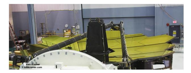
Gold coated primary mirrors newly exposed on spacecraft structure of NASA's James Webb Space Telescope inside the massive clean room at NASA's Goddard Space Flight Center in Greenbelt, Maryland on May 3, 2016. Aft optics subsystem stands upright at center of 18 mirror segments between stowed secondary mirror mount booms. Credit: Ken Kremer/kenkremer.com
