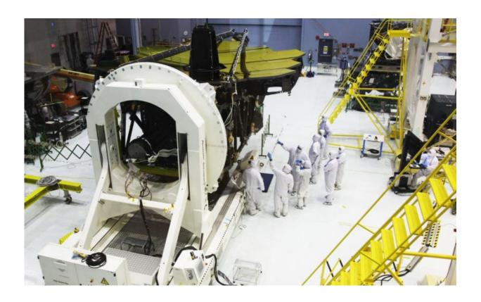
All 18 gold coated primary mirrors of NASA's James Webb Space Telescope are seen fully unveiled after removal of protective covers installed onto the backplane structure, as technicians work inside the massive clean room at NASA's Goddard Space Flight Center in Greenbelt, Maryland on May 3, 2016. The secondary mirror mount booms are folded down into stowed for launch configuration. Credit: Ken Kremer/kenkremer.com
