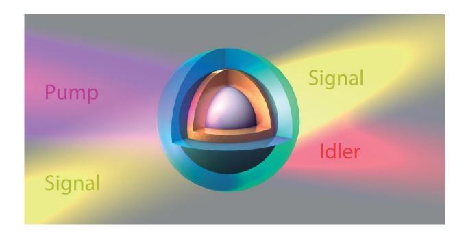
Rice University's new light-amplifying nanoparticle consists of a 190-nanometer diameter sphere of barium tin oxide surrounded by a 30-nanometer-thick shell of gold. Credit: Alejandro Manjavacas /Rice University
