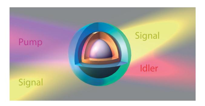
Rice University's new light-amplifying nanoparticle consists of a 190-nanometer diameter sphere of barium tin oxide surrounded by a 30-nanometer-thick shell of gold. Credit: Alejandro Manjavacas /Rice University
