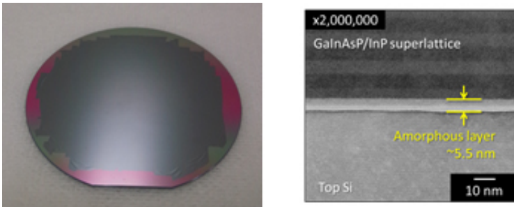
Figure 1. Optical microscope and SEM images of GaInAsP/SOI hybrid wafers.
