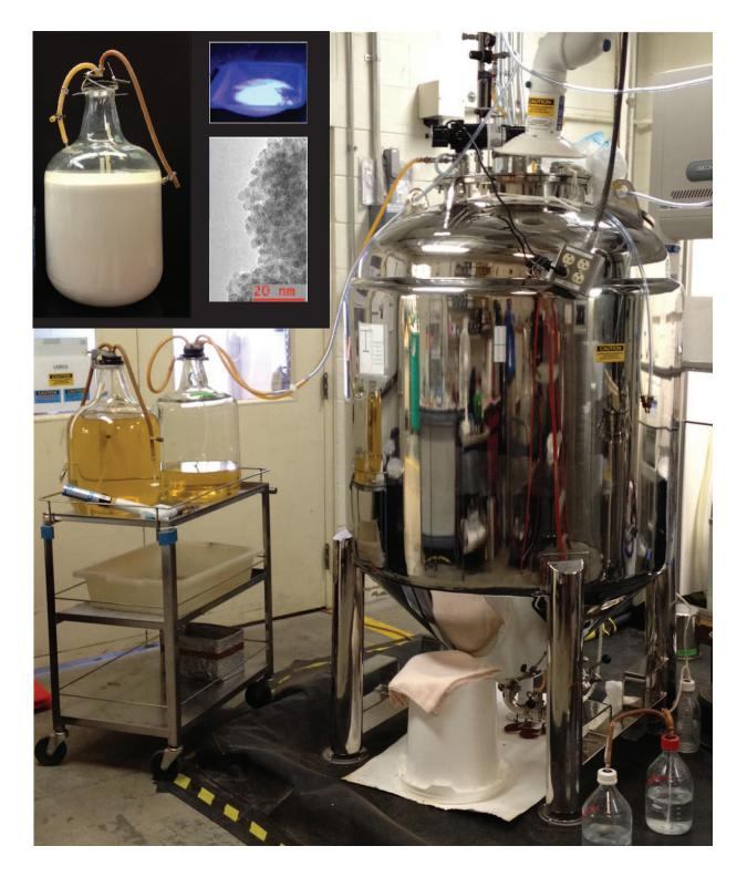
Using this 250-gallon reactor, ORNL researchers produced three-fourths of a pound of zinc sulfide quantum dots, shown in the inset. Credit: ORNL
