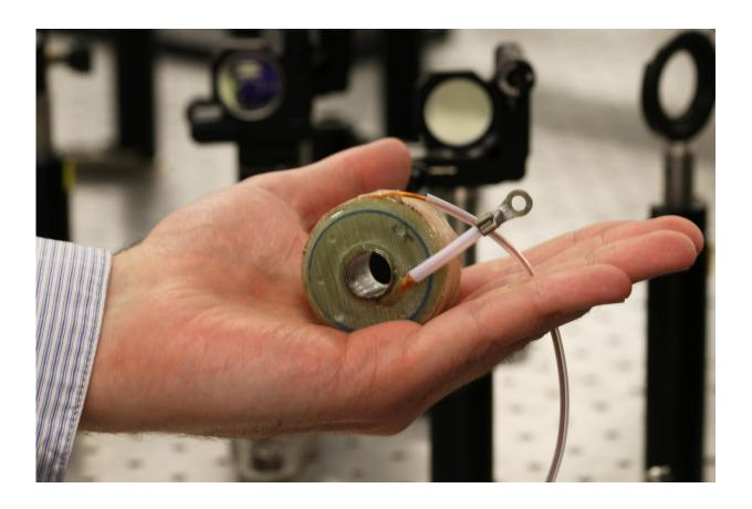
The magnetic coil at the heart of the system was developed by Professor Hiroyuki Nojiri at the Institute of Materials Research, Tohoku University (Japan). It produces a pulsed magnetic field of up to 30 Tesla. Credit: S. Hammersley, The University of Manchester
