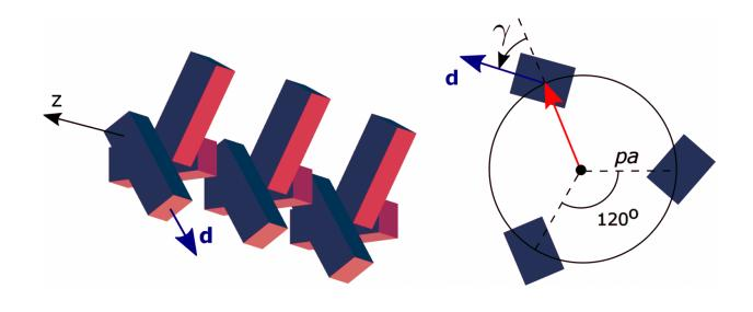
Structure of the helical chiral supercrystal. Credit: ITMO University
