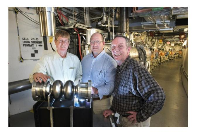
Brookhaven Lab staff members (left to right) James Rose, John Gosman, and William Gash with one of the two electron bunch–lengthening radio-frequency cavities that will be installed at the National Synchrotron Light Source II (NSLS-II). By reducing the number and intensity of collisions between electrons circling the NSLS-II electron storage ring, these cavities will help prevent electron beam loss and thus extend the lifetime of the beams used to conduct experiments.
