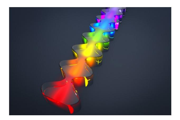
An artist's embellishment of an image of the "gain medium" used to produce terahertz frequency combs. The different colors indicate that different wavelengths of oscillating terahertz radiation travel different distances through the medium, which has a different refractive index for each of them. Credit: Yan Liang/L2Molecule.com
