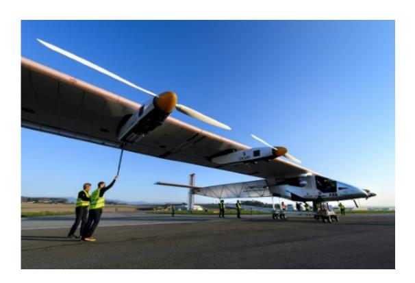
The Solar Impulse 2 has wings wider than those of a Boeing 747 and contains 17,000 solar cells that power its propellers
