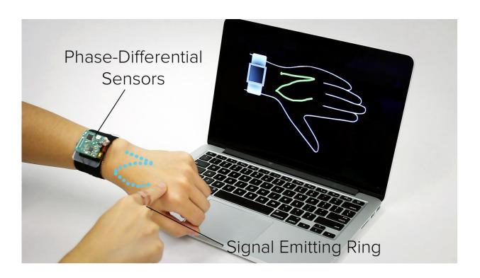
Carnegie Mellon University's SkinTrack enables users to turn their skin into a touchpad for controlling smartwatches. User wears only a signal-emitting ring, which propagates electromagnetic waves in the skin that can be localized with sensors worn on the wrist. Credit: Future Interfaces Group, Carnegie Mellon University
