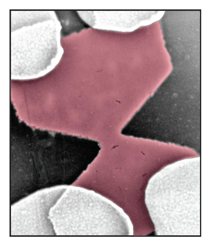
Scanning electron microscopy (SEM) image of graphene nanoconstriction: graphene material is shown in red, 4 metal electrodes are also seen. Credit: B. Terrés, L. A. Chizhova, F. Libisch, J. Peiro, D. Jörger, S. Engels, A. Girschik, K. Watanabe, T. Taniguchi, S. V. Rotkin, J. Burgdörfer, C. Stampfer
