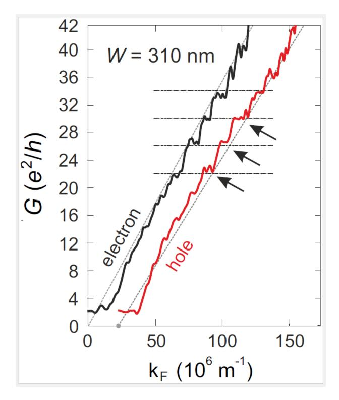
This graph shows electrical conductance, G, of electrons (black) and holes (red) in graphene nanoconstriction (shown in SEM image), as a function of electron/hole wave vector (momentum) showing characteristic steps
