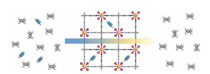
Ethylene (on left in gray) is usually contaminated with acetylene (blue), which can ruin the process that creates the polyethylene used in most plastic. SIFSIX metal-organic frameworks (center) can capture the acetylene efficiently, leaving pure ethylene (right). Credit: Zhou / NIST
