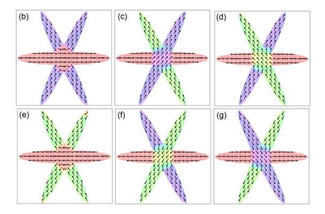
Six magnetic configurations generated by simulations. Credit: Telepinsky et al. ©2016 AIP Publishing
