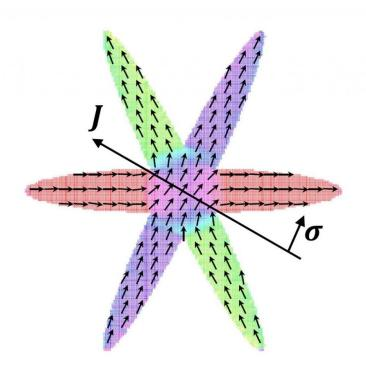
By arranging magnetic film into a pattern of three crossing ellipses, researchers demonstrated six magnetic configurations are possible in the overlapping region. Credit: Telepinsky et al. ©2016 AIP Publishing
