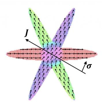
By arranging magnetic film into a pattern of three crossing ellipses, researchers demonstrated six magnetic configurations are possible in the overlapping region. Credit: Telepinsky et al. ©2016 AIP Publishing
