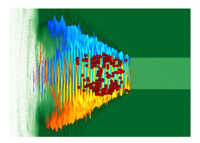
Calculated electron density (green) and magnetic field strength (yellow-orangeblue) inside a structured plastic target 300 femtoseconds after being irradiated with an intense laser pulse from the left-hand side. The red dots indicate locations where photons with energy greater than 10 MeV were emitted in this simulation. The photons (not shown) exit to the right. Credit: A. V. Arefiev, D. J.
