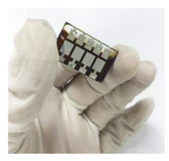
A perovskite photovoltaic cell that was produced without using the conventional thermal drying process offered better performance. Credit: A\*STAR Institute of Materials Research and Engineering
