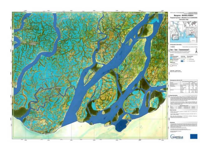
Following the activation of the Copernicus Emergency Mapping Service on 22 May 2016, data from Sentinel-1A's radar scan on 23 May were made available to the service in rush mode. The data were then used to create this map of Barguna showing over 85 000 hectares of flooded areas in light blue. Credit: Copernicus Service information (2016) / Copernicus EMS / e-GEOS
