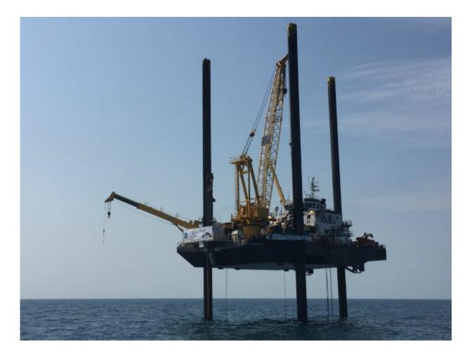
The drilling platform L/B Myrtle whihe is being used in the Gulf of Mexico. Credit: ECORD and IODP
