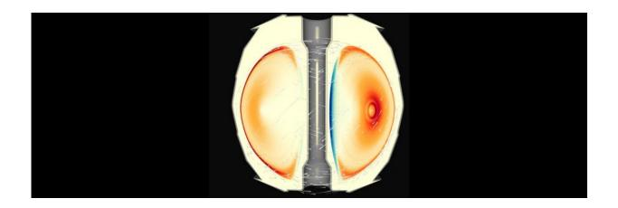
Simulation shows trapped electrons at left and passing electron at right that are carried in the bootstrap current of a tokamak. Credit: Kwan Liu-Ma, University of California, Davis
