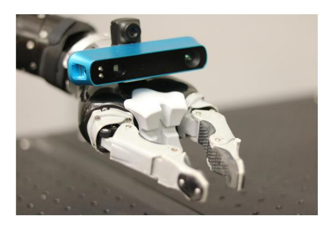
Researchers at Carnegie Mellon University's Robotics Institute have shown that a camera attached to a robot's hand can rapidly create a 3-D model of its environment and also locate the hand within that 3-D world. Credit: Personal Robotics Lab
