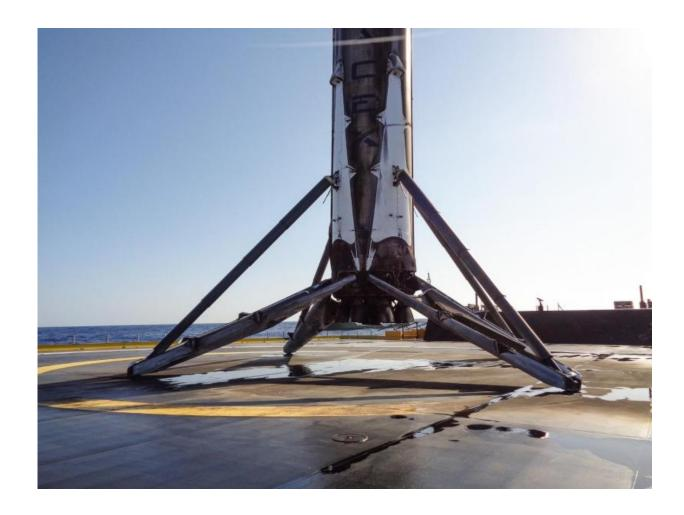
Base of Recovered Falcon 9 first stage with landing legs after drone ship landing following SpaceX launch of JCSAT-14 on May 6, 2016 from Space Launch Complex 40 at Cape Canaveral Air Force Station, Fl. Credit: SpaceX
