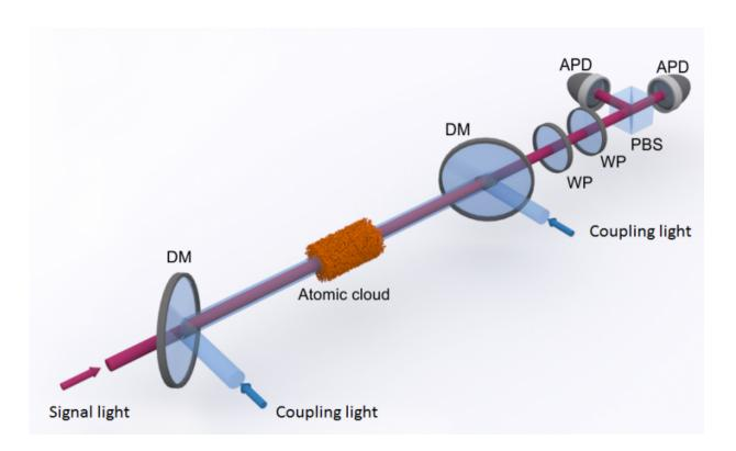
A cloud of cold atoms is illuminated with red signal light and blue coupling light. The light pulses are superimposed on dichroic mirrors (DM). With wave plates (WP), a polarizing beam splitter (PBS), and avalanche photodiodes (APD) the polarization of the transmitted signal light is determined. Credit: MPQ, Quantum Dynamics Division
