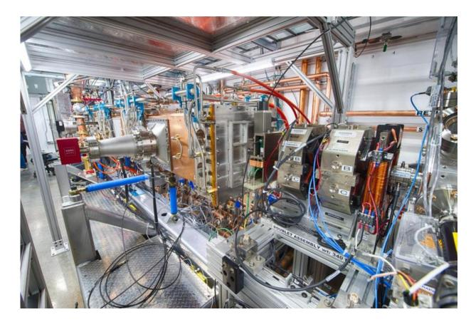
The RFQ is undergoing tests at the Cryomodule Test Facility at Fermilab. Credit: Reidar Hahn
