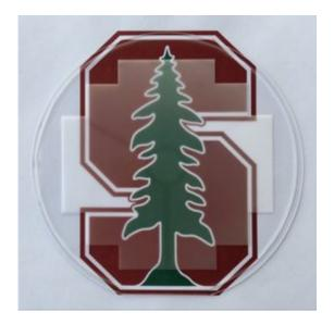
The Stanford logo is clearly visible under the etched silica layer, demonstrating its transparency. Credit: Linxiao Zhu/Stanford
