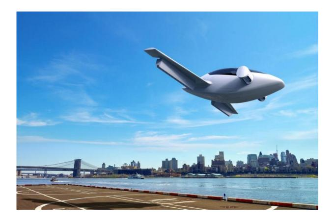
ESA BIC Bavaria start-up Lilium is developing a two-seater electric powered plane for personal use. Although taking off and landing like a helicopter, by rotating its engines it also functions as a very efficient fixed-wing aircraft that can travel at up to 400 km/h and have a range of 500 km. Credit: Lilium
