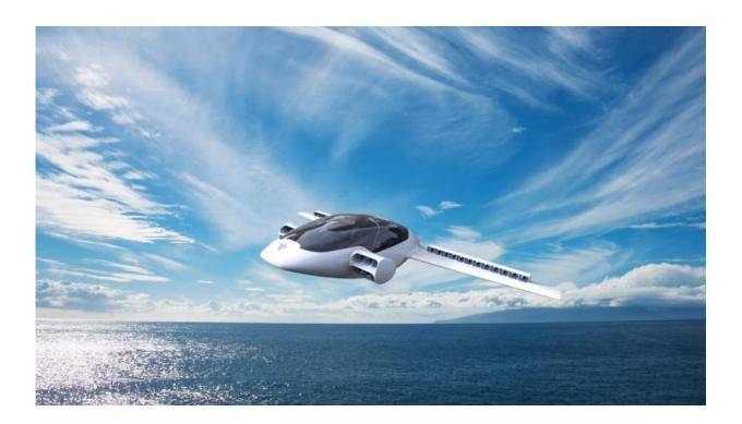
ESA BIC Bavaria start-up Lilium is developing a two-seater electric powered plane for personal use. Although taking off and landing like a helicopter, by rotating its engines it also functions as a very efficient fixed-wing aircraft that can travel at up to 400 km/h and have a range of 500 km. Credit: Lilium
