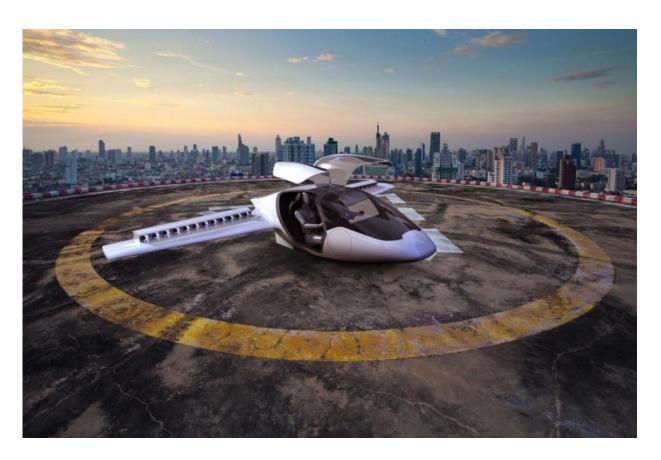
The electric aircraft under development by ESA BIC Bavaria start-up Lilium needs only an open flat area of about 15x15 m for vertical takeoff and landing. The environmentally friendly aircraft is planned to be available from 2018. Credit: Lilium
