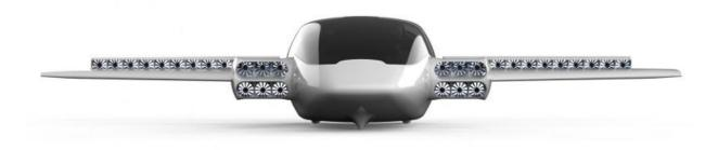
Entirely electric, the Lilium plane is much quieter during takeoff than helicopters thanks to its ducted fan engines. The fans are positioned vertical during takeoff and landing, and turned horizontal for flying to make the plane a very efficient fixed-wing aircraft that can travel at up to 400 km/h. Credit: Lilium
