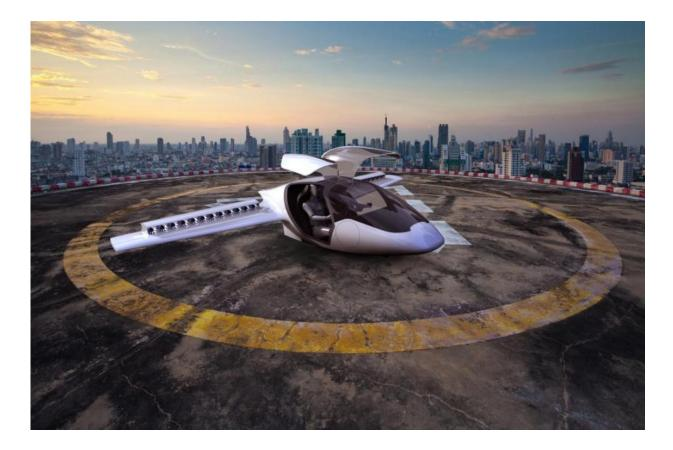
The electric aircraft under development by ESA BIC Bavaria start-up Lilium needs only an open flat area of about 15x15 m for vertical takeoff and landing. The environmentally friendly aircraft is planned to be available from 2018. Credit: Lilium
