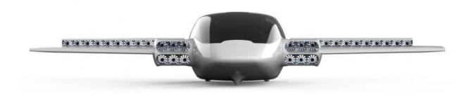
Entirely electric, the Lilium plane is much quieter during takeoff than helicopters thanks to its ducted fan engines. The fans are positioned vertical during takeoff and landing, and turned horizontal for flying to make the plane a very efficient fixed-wing aircraft that can travel at up to 400 km/h. Credit: Lilium
