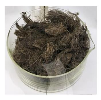
Biomass such as this waste from palm oil production could replace petrochemicals for making nylon. Credit: A\*STAR Institute of Chemical and Engineering Sciences
