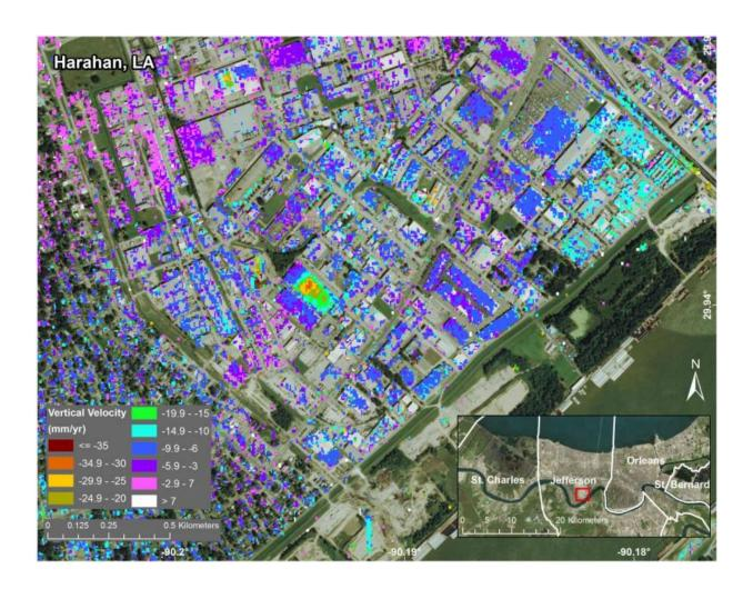
Subsidence in Jefferson Parish, Louisiana, from June 2009 to July 2012, as seen by NASA's UAVSAR instrument. The measured displacements are a combination of movement of the ground and of individual structures. The inset at lower right shows the parish location within Greater New Orleans. Credit: NASA/JPL-Caltech, Esri
