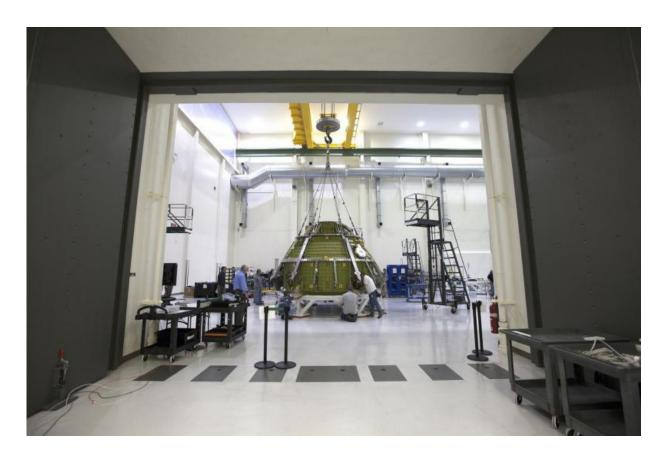
Lockheed Martin engineers and technicians prepare the Orion pressure vessel for a series of tests inside the proof pressure cell in the Neil Armstrong Operations and Checkout Building at NASA's Kennedy Space Center in Florida. Credit: NASA/Kim Shiflett
