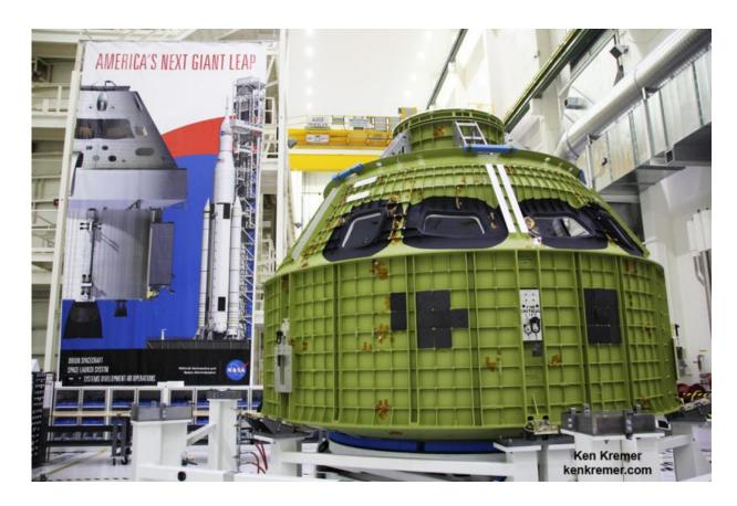
Orion crew module pressure vessel for NASA's Exploration Mission-1 (EM-1) is unveiled for the first time on Feb. 3, 2016 after arrival at the agency's Kennedy Space Center (KSC) in Florida. It is secured for processing in a test stand called the birdcage in the high bay inside the Neil Armstrong Operations and Checkout (O&C) Building at KSC. Launch to the Moon is slated in 2018 atop the SLS rocket. Credit: Ken Kremer/kenkremer.com
