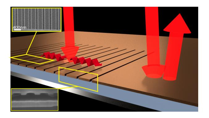
When light falls on a very thin, uniform layer almost all of it is reflected (right-hand arrows). By etching thin grooves in the film, the light is directed sideways and almost all of it is absorbed (left-hand arrows) even though the amount of material is very small. Insets show electron micrographs of the structuring. The absorbing layer is only  $0.041~\mu m$  thick. Credit: Dr Thomas P. White, Australian National University.
