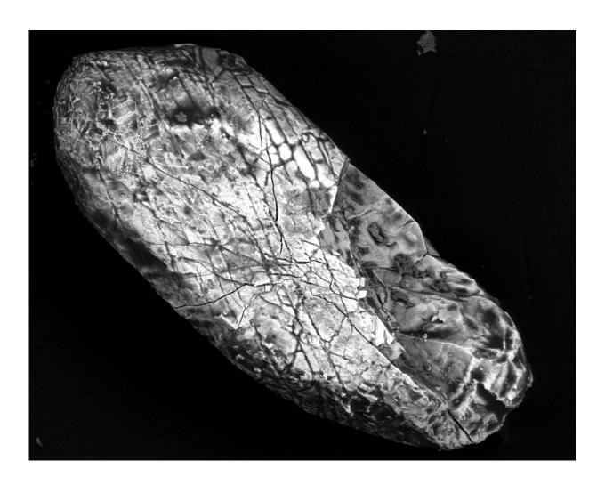
Scanning electron microscope image of a shock-metamorphosed zircon from the Sudbury impact crater, Ontario, Canada. The parallel planar fractures are caused by the extreme conditions of the impact itself while the anastomosing cracks represent later damage. The zircon is less than 0.1 mm wide. Credit: Gavin Kenny, Trinity College Dublin, in *Geology*.
