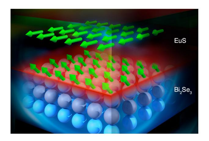
Illustration showing structure of Bi2Se3-EuS bilayer film. On the top layer the depth profile of the magnetization vector distribution of Eu atoms is represented by green arrows. The light purple spheres represent Bi2Se3 interfacial layers magnetized in close proximity to EuS FMI. Credit: ORNL/Jill Hemman
