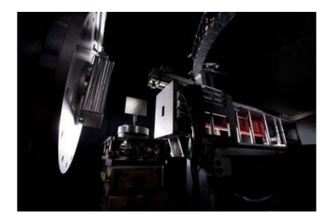
The ILL's D17 reflectometer was used to investigate the interactions of different forms of Aß with this synthetic membrane, imitating the outside layer of neurons found in the brain. Credit: Institut Laue-Langevin (ILL)
